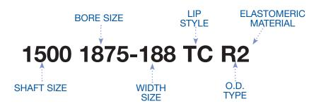
**Shaft Size** - The first four digits in the part number describe the nominal shaft size to three decimal places. If the shaft size is greater than 10 inches, five digits will be used for this portion of the part number.
